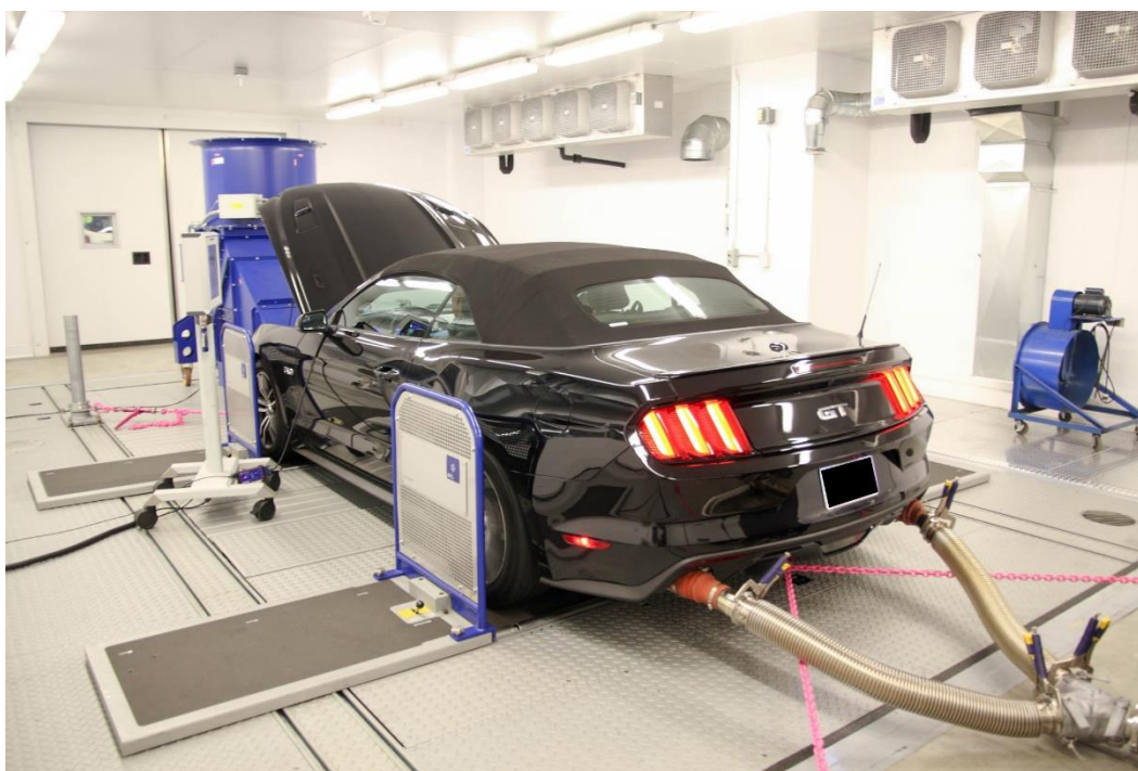
Figure 9: 2017 Ford Mustang GT on Dynamometer
