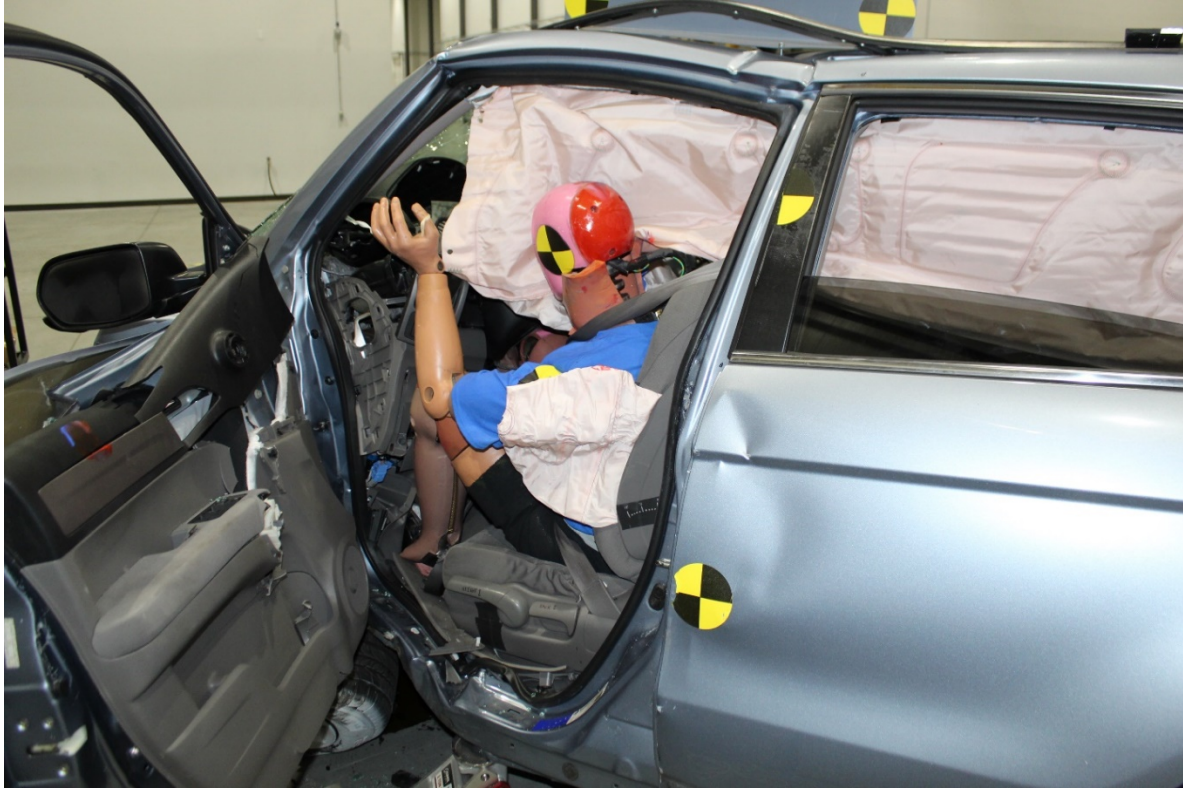
Deformed vehicles and dummy on driver seat
