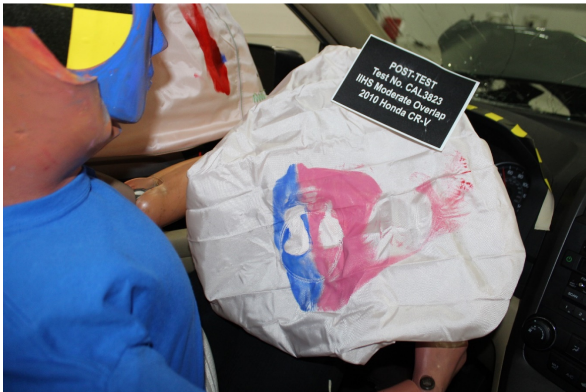
Deployed airbag with paint mark from dummy's head
