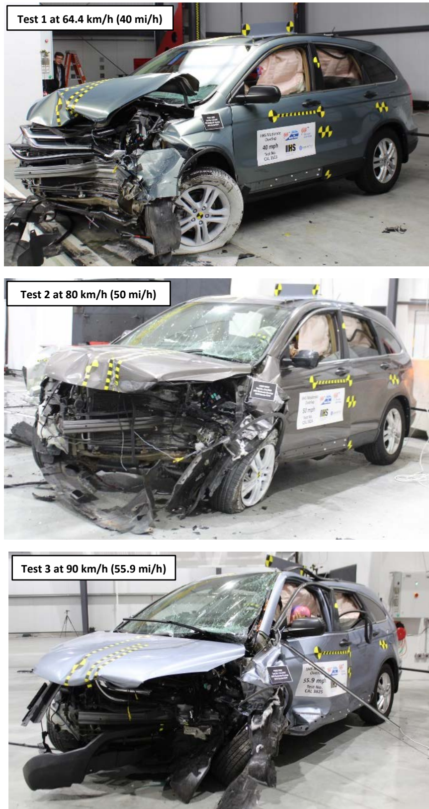
Figure 20. Visual comparison of vehicle exterior between the three tests
