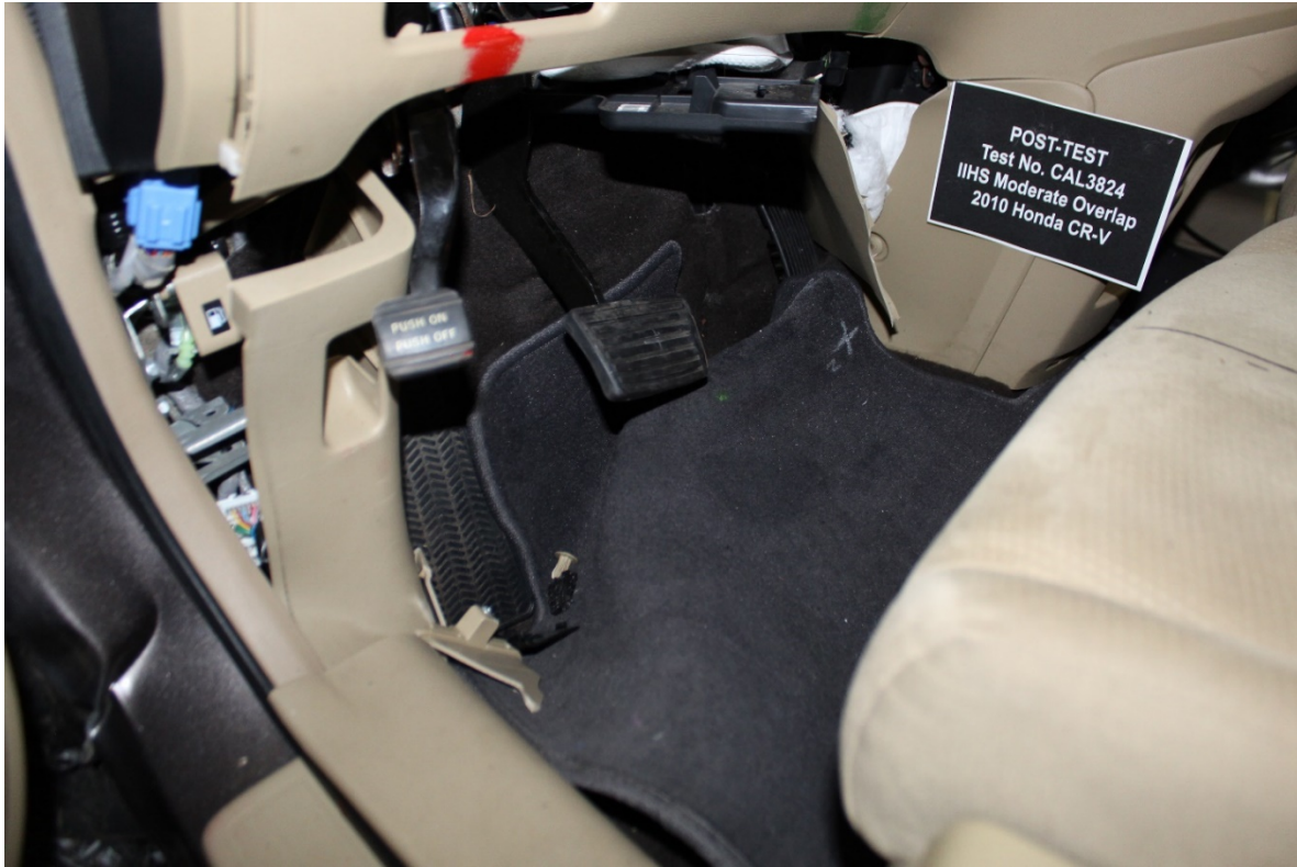
Footwell intrusion after displacing the dummy
