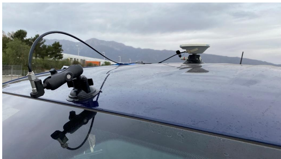
Figure 8: Rain system injector nozzle and mount. Image source: AAA
