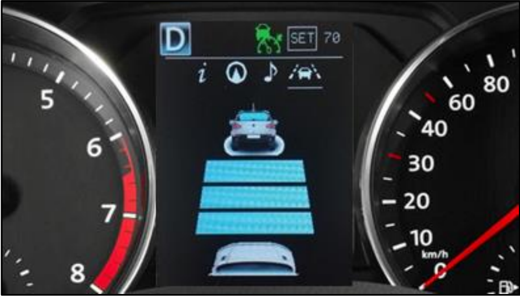
Figure 4. Close Up of ACC Interface
