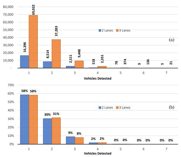
Figure 18. Distribution of the number of detected vehicles (1-7) in each frame by the number of lanes: (a) the raw counts of frames with the corresponding number of vehicles; (b) the percentage of frames with the corresponding number of vehicles.
