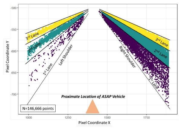
Figure 12. Lane positions of vehicles detected in every frame
