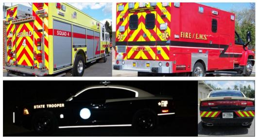
Figure 1. Examples of responder vehicles with high conspicuity markings. (USDOT, 2019)
