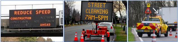
Figure 3. Permanent VMS, portable VMS, and truck-mounted VMS. (Sources: commons.wikimedia.org; 4directionssigns.com; and ebovanweel.com)
