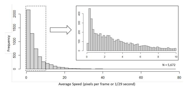
Figure 17. Distribution of average speed at the vehicle trajectory level. The inset figure magnifies the values at lower speeds.
