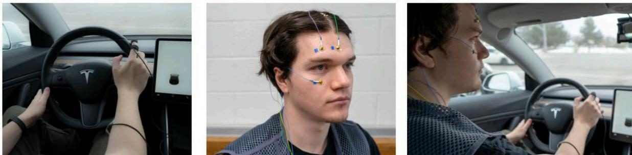
*Figure 3. The DRT vibrotactile stimulus and microswitch response button setup (left), EEG electrode setup (middle), and the combination of the two while driving (right).*
