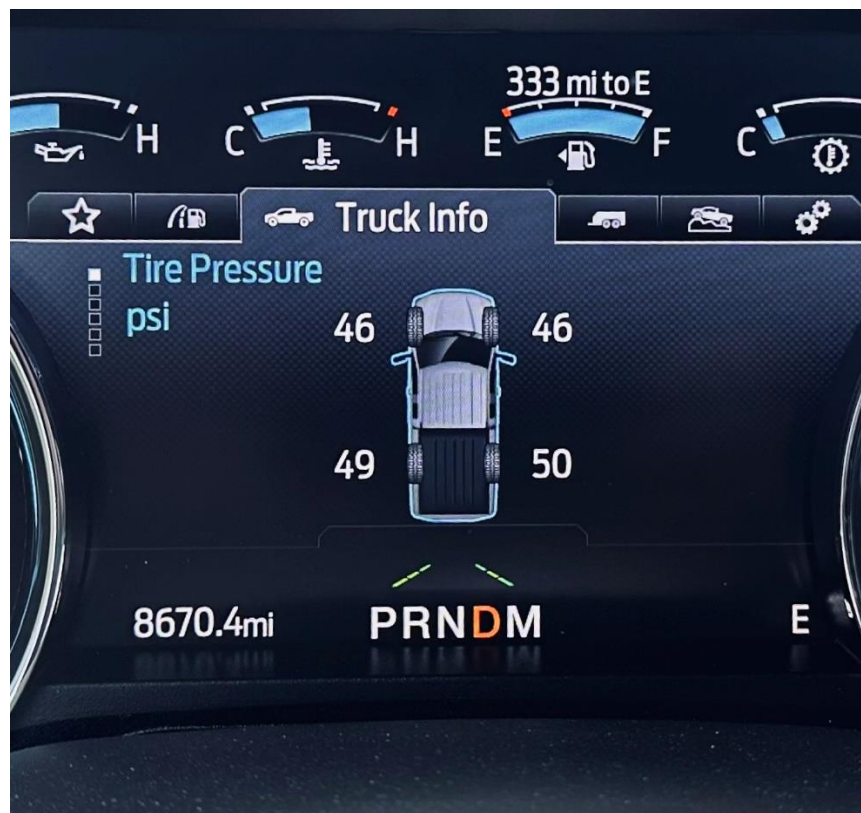
Figure 11: 2022 Ford F-250 display at 75 percent of placard pressure. Image Source: AAA.
