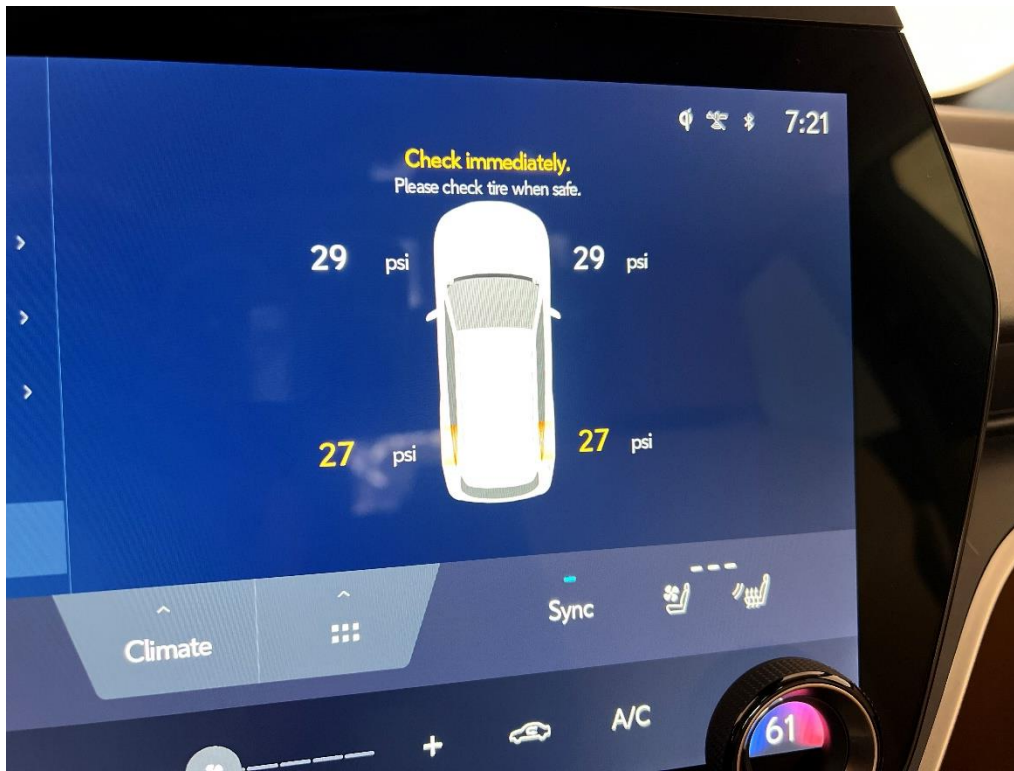
Figure 16: 2023 Lexus RZ450e display at 75 percent of placard pressure. Image Source: AAA.
