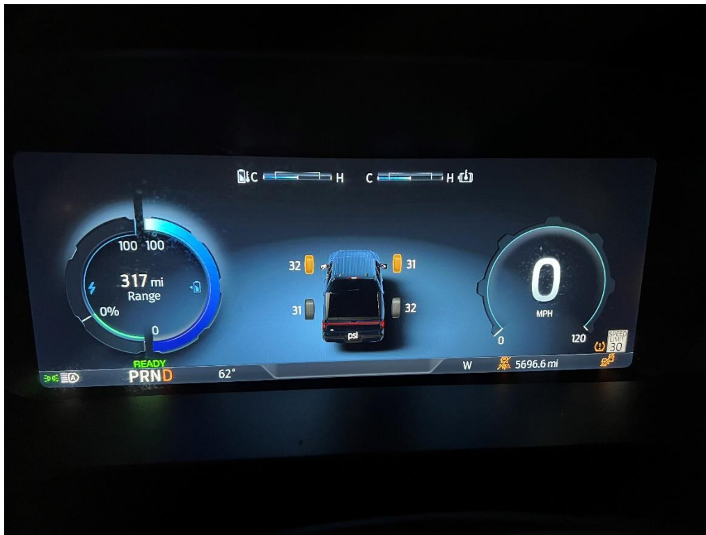
Figure 10: 2022 Ford F-150 Lightning display at 75 percent of placard pressure. Image Source: AAA.
