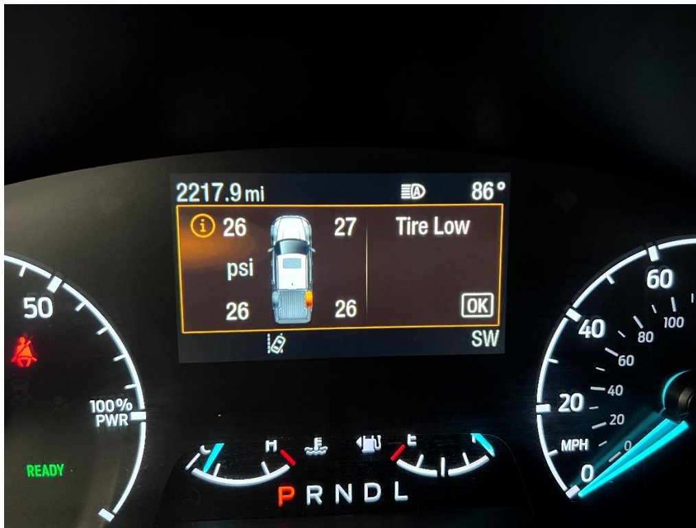
Figure 12: 2023 Ford Maverick display at 75 percent of placard pressure. Image Source: AAA.
