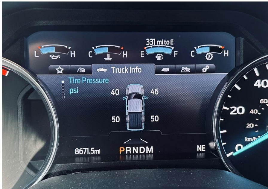
Figure 7: 2022 Ford F-250 with left front tire inflated to 65 percent of placard pressure. Image Source: AAA.
