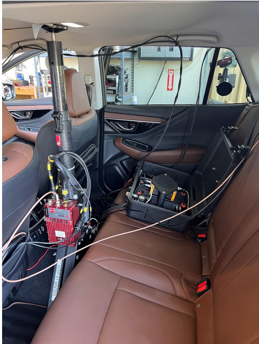
Figure 9: Oxford Precision GPS and DEWESoft Data Logger Setup in Vehicle. Image Source: AAA Inc.
