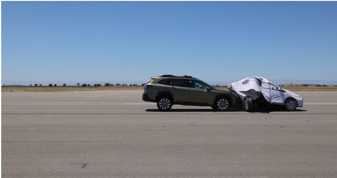
Figure 38: Late Model Subaru Outback collision with Soft Car at 55 mph. Image Source: AAA Inc.
