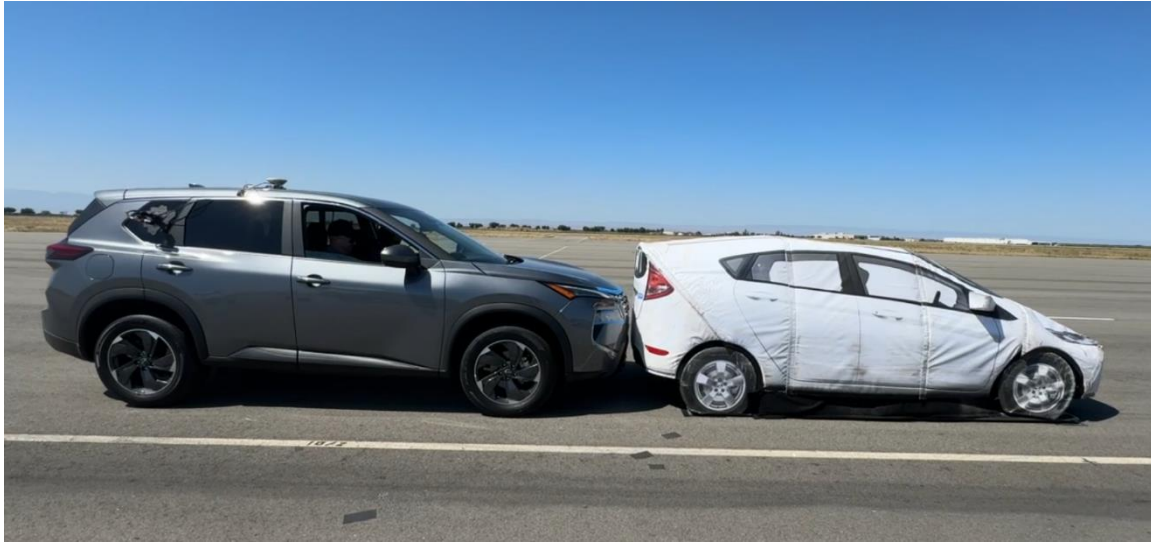
Figure 34: Late Model Nissan Rogue 45-mph Run 4—Close Stop Event. Image Source: AAA Inc.
