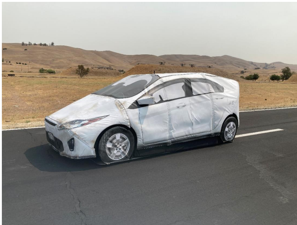
Figure 11: DRI Soft Car 360° on Static Base. Image Source: AAA
