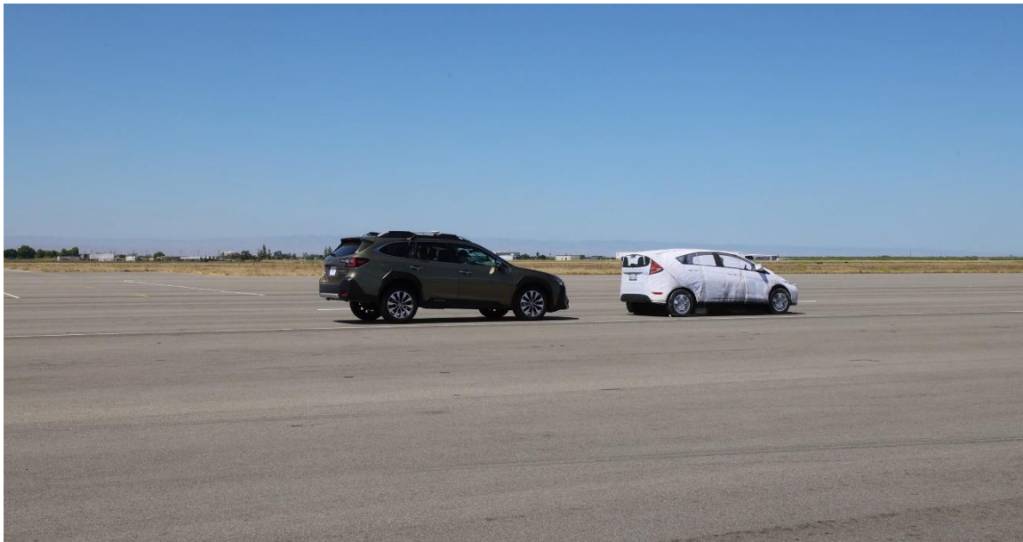
Figure 19: Late Model Subaru Outback braking at 12 mph. Image Source: AAA Inc.
