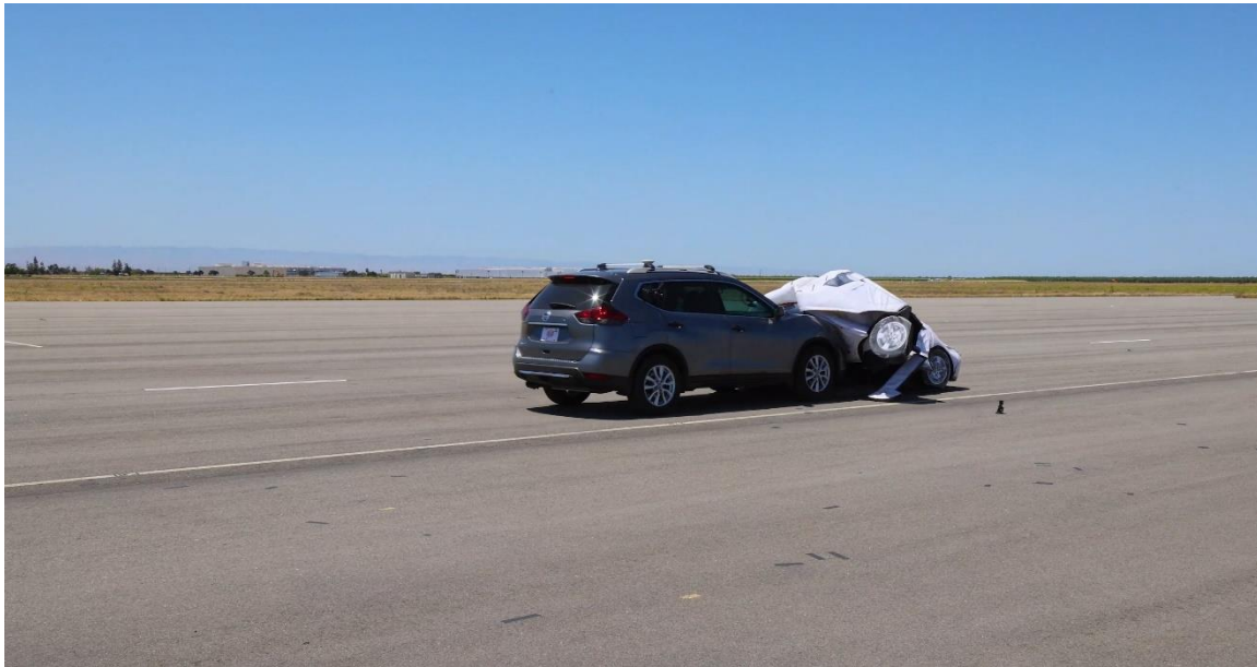
Figure 22: Early Model Nissan Rogue impact at 25 mph. Image Source: AAA Inc.
